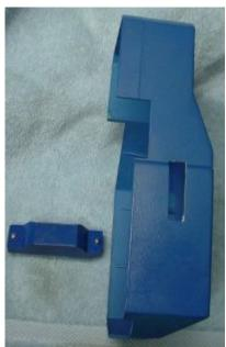
This is the slot in the cover required to accommodate the fine feed module. The edge of my slot is 1 inch from the open side but yours may differ so Dremel it as needed, trying for fit frequently. A small cover could be added over the exposed gear per the example next to the gear cover.
