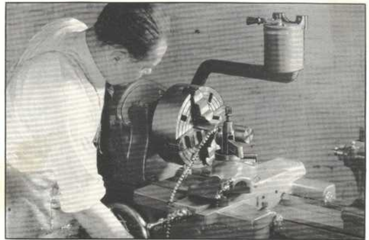
Fig. 148. Machining a Shaft in an Independent Chuck
