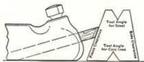
Fig. 54-B. Checking Front Clearance
