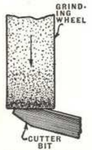
Fig. 58. Grinding Right Side of Cutter Bit
