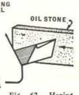
Fig. 62. Honing the Cutting Edge of Cutter Bit with an Oil Stone
