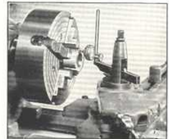
Fig. 155. Testing Face of Work with Dial Indicator for Wobble
