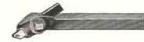
Fig. 50. Right Hand Tool Holder
