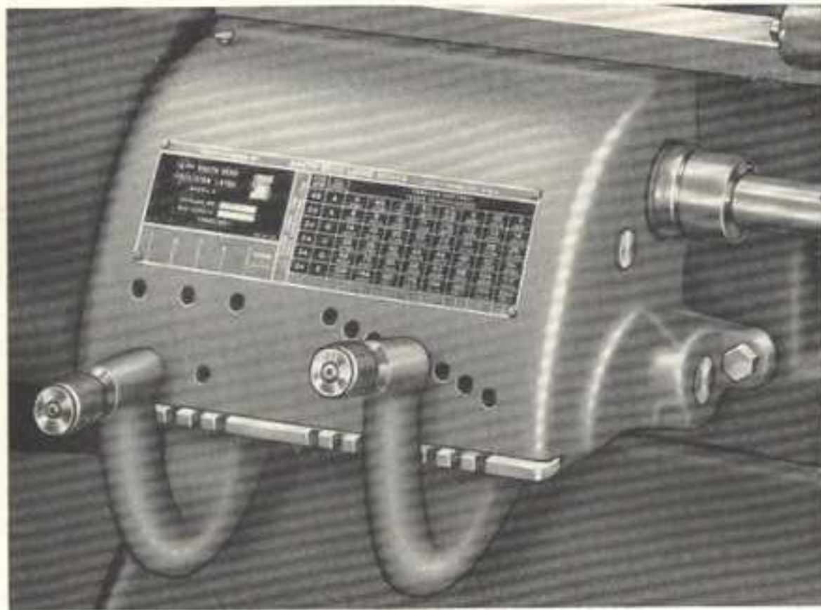
Fig. 7. A Modern Quick Change Gear Box
