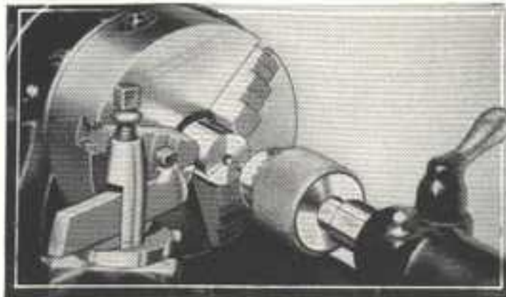
Fig. 125. Drilling a Center Hole with Stock Held in Lathe Chuck and Drill in Tailstock Spindle Chuck
