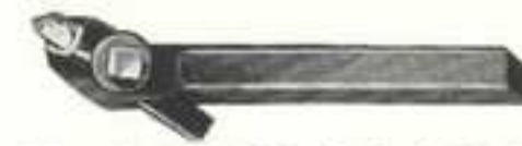
Fig. 48. Left Hand Tool Holder
