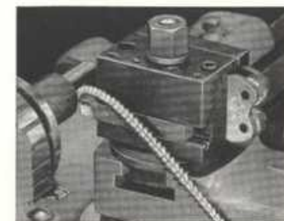
Fig. 88A. Machining a Steel Shaft at High Speed with Carbide Tipped Cutting Tool
