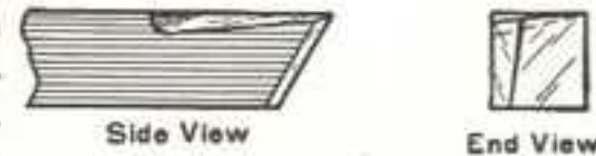
Fig. 64. Detail of Roughing Tool
