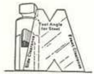
Fig. 54-A. Checking Side Clearance
